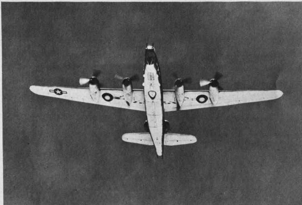
The new Liberator's lines are more familiar when seen from below. Contrast between its graceful wing and the rectangular fuselage still marks the plane as descendant of the B-24.
